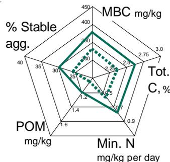
The NI and HI systems have the lowest soil quality, as shown by the smaller area encompassed by the colored lines. The areas encompassed by solid lines (4-yr rotations) are much larger than those of the dashed line (2-yr rotations), showing that the NI and HI systems had greater positive responses to the extended rotations than did the RI and OI systems.
